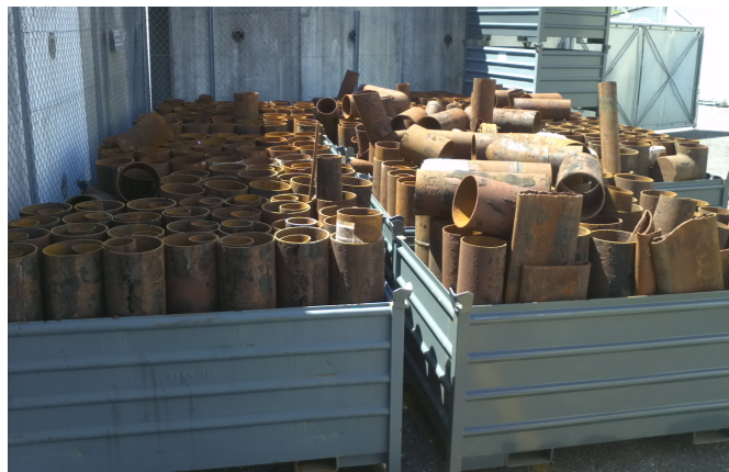
Figure 1.2: The PS pipes after the cutting process.
