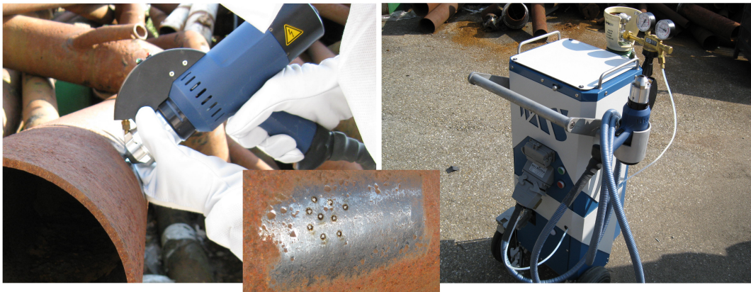
Figure 5.3: Optical Emission Spectroscopy analyser (PMI-Master pro).
