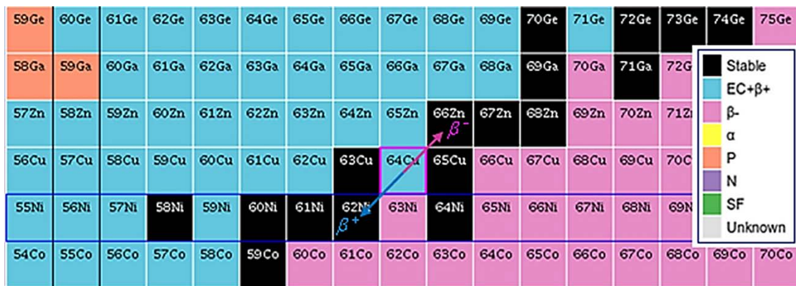
Fig. 2.4: Decay modes of {}^{64}_{29}\text{Cu} . (Retrieved and adapted from [Sonzogni, 2013].)
