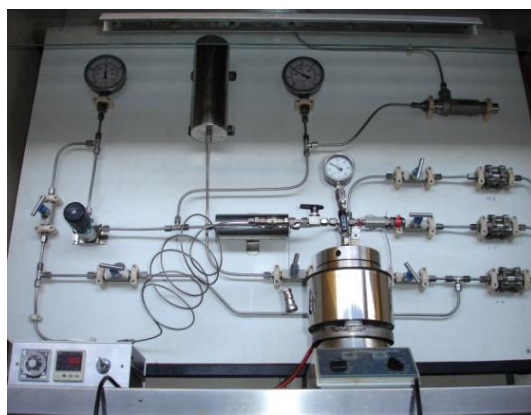
Figure 5.1 – High-pressure system for catalytic hydroformylation, in the Chemistry Department, University of Coimbra.
