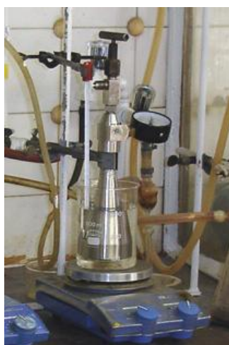
Figure 5.4 – Autoclave for high-pressure catalytic aminocarbonylation reactions in the Department of Inorganic Chemistry, University of Pécs.
