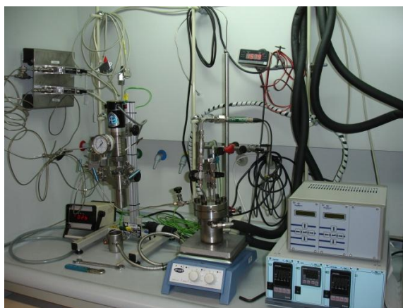
Figure 5.3 – High-pressure system for catalytic hydrovinylation, in the Department of Inorganic Chemistry, University of Barcelona.
