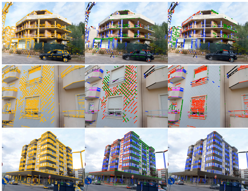
Figure 4.11: (Left) extracted edges, and (right) detection results. In each example (row) we detected 2 groups of orthogonal triplets with the blue VD in common. The VD in magenta (row 3) was detected but (incorrectly) not assigned to any triplet.
