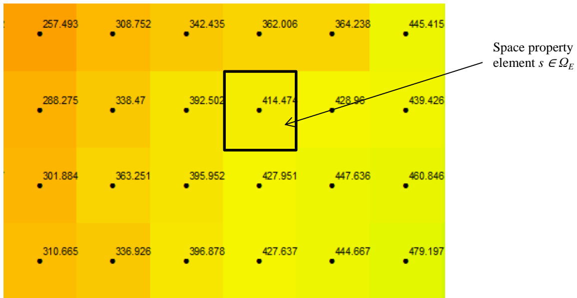
Figure 5-2 Zoom of a 1,200 * 800 \text{ m}^2 rectangle of the search area: grid elevation data and the corresponding discretization space property elements. Elevation data in meters.
