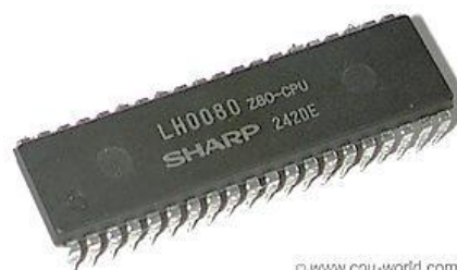
Figure 1-1. Zilog Z80 - 8-bit microprocessor designed and sold by Zilog from July 1976. [7]
