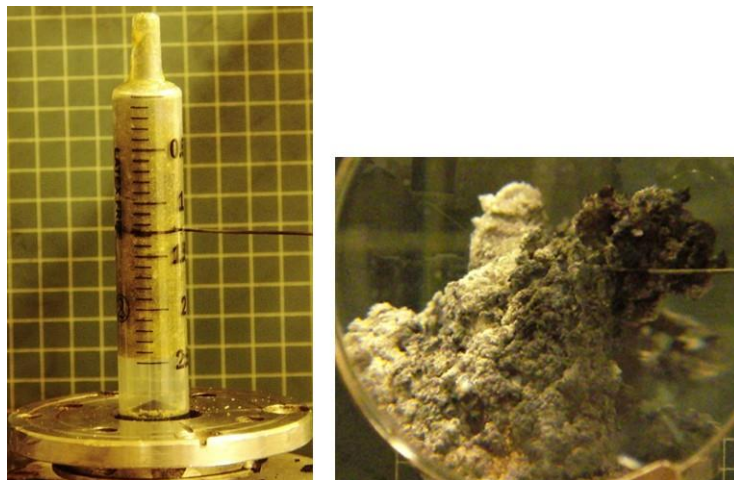
Figure 134: Mixture n°. 3.2 prepared for a cigar burning test (left) and its residues of combustion (right).
