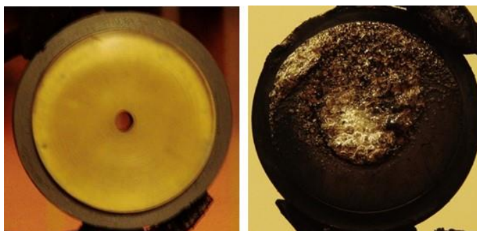
Figure 133: Disk of mixture n°. 4.1. Image on the left shows the fresh mixture on the disk. Image on the right shows the disk after the combustion.
