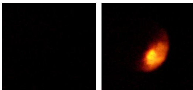
Figure 79: Frames which shows the moment before explosion one (at left) and the first appearance of explosion one (at right). The measurement of the area was made at right image.
