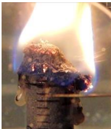
Figure 124: Flame of combustion of mixture n°. 3.4 used for measurements of fundamental flame velocity.
