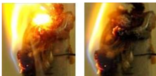
Figure 98: Frames used to study the velocity of propagation of explosion in mixture n°. 3.1.
