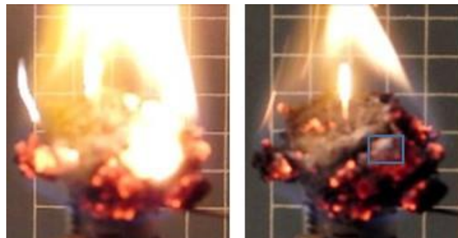
Figure 106: Frames used to study the velocity of propagation of explosion in mixture n°. 3.2.
