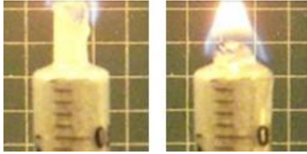
Figure 113: Frames used to study the velocity of the propagation of the flame on PMMA. The initial position is image on the left, final position the image on the right.
