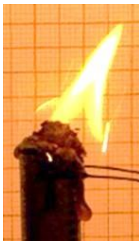
Figure 82: Flame of combustion of mixture n°. 1.8 on a cigar burning test
