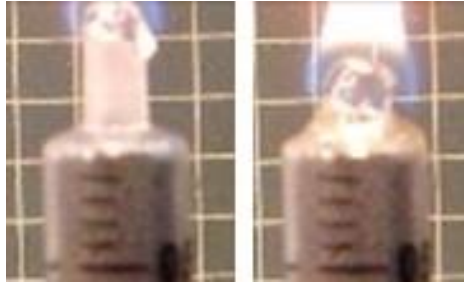
Figure 121: Frames used to study the velocity of the propagation of the flame on PMMA. The initial position is image on the left, final position the image on the right.
