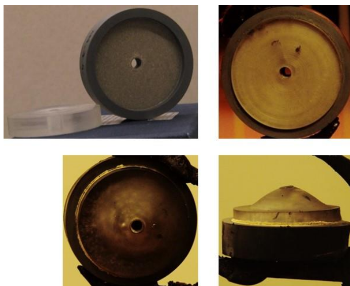
Figure 116: Disk of mixture n°. 3.3. Images on the top shows the fresh mixture on the disk. Images on the bottom shows the disk after combustion.
