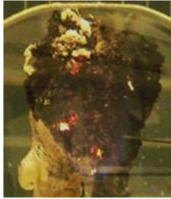
Figure 129: Aspect of the mixture n°. 4.1 during its combustion on a cigar burning test
