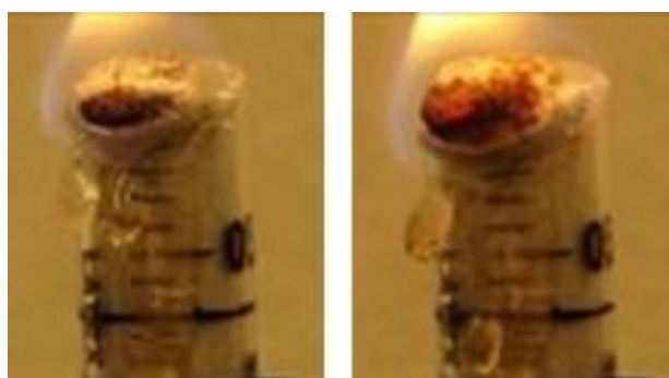
Figure 97: Frames used to study the velocity of the propagation of the flame on PMMA. The initial position is image on the left, final position the image on the right.
