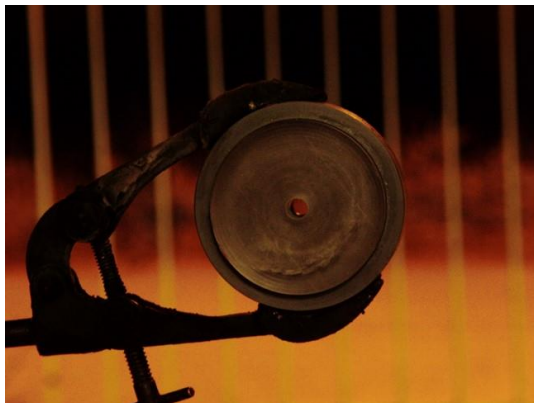
Figure 60: vertical experiment set-up for disk burning test
