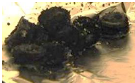
Figure 71: Mixture n°. 1.5 prepared for a cigar burning test (left) and its residues after combustion (right)
