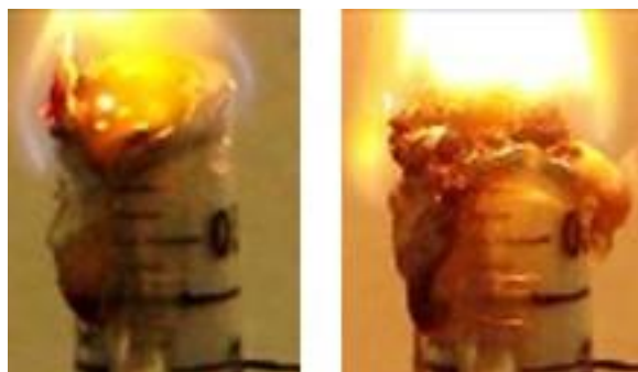
Figure 99: Frames used to study the velocity of flame propagation in the mixture n°. 3.1. The frame at the left is correspondent to the initial position, and the frame at right, the final position.
