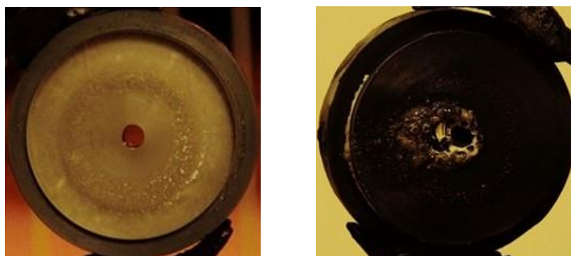
Figure 100: Disk of mixture n°. 3.1. Image on the left shows the fresh mixture on the disk. Image on the right shows the disk after the combustion.
