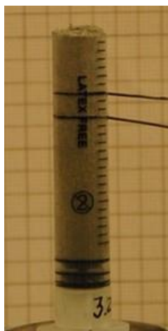
Figure 71: Mixture n°. 1.5 prepared for a cigar burning test (left) and its residues after combustion (right)
