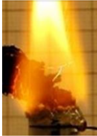
Figure 72: Flame of combustion of mixture n°.1.5 on a cigar burning test.
