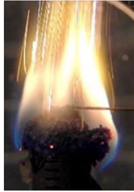
Figure 120: Aspect of the flame during the combustion of the mixture n°. 3.4 on a cigar burning test
