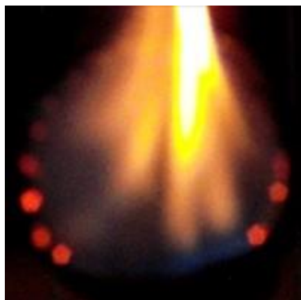
Figure 140: Combustion of disk with mixture n°. 4.2 where it is possible to see the PMMA's flame and hotspots of the mixture.
