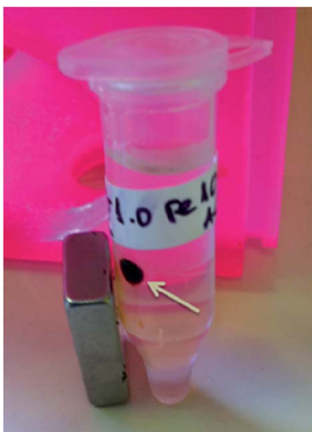
Fig. 9 Demonstration of nanomagnetogel accumulation under an external magnetic field (overnight).
