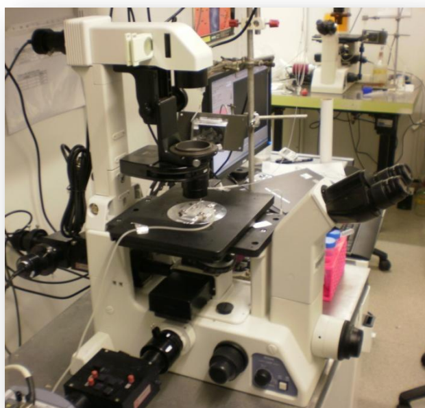
Figure 22 - Nikon Eclipse TE 300 microscope (left) and gravity perfusion system with VC-6 (right) used for imaging studies.
