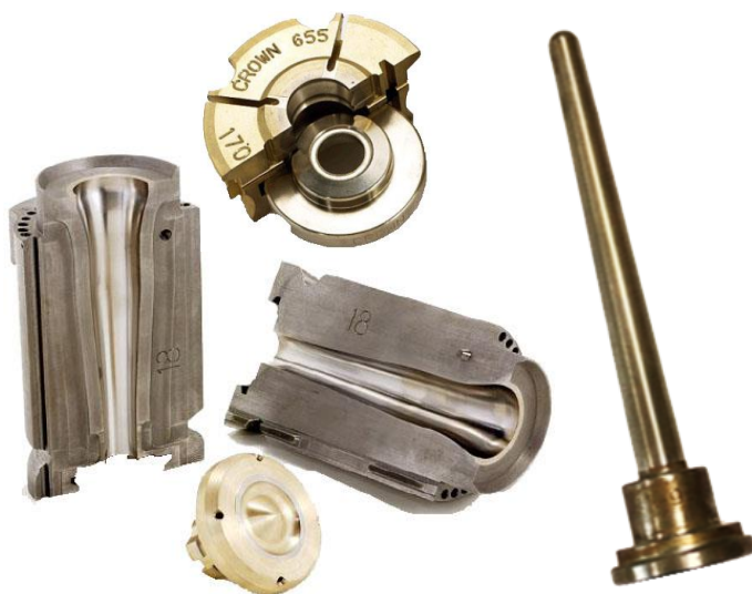
Figure 2.1 - Components used in glass containers production.
