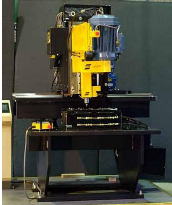
Figure 2.9 – Dedicated FSW machine – FSW Legio™ (ESAB, 2014).
