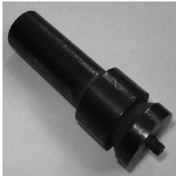
Figure 2.2 – Conventional FSW tool with large shoulder (Source: (Aydin, 2010)).
