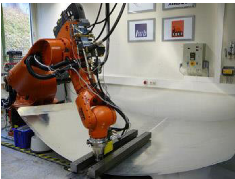
Figure 2.11 – Articulated arm robot performing FSW (TUM, 2014).
