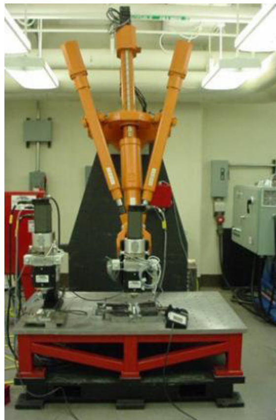
Figure 2.12 – Parallel-kinematic robot (Tricept) performing FSW (PKM TRICEPT, 2014).
