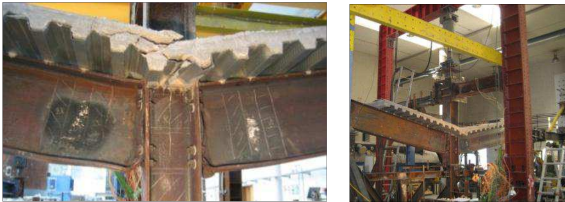
Figure 3.35: Final deformation of the tested structure (test 6)
