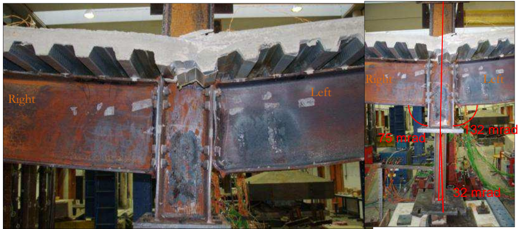
Figure B.16: Final deformation of the sub-frame under sagging bending moment (back view / test 3 – 700°C and no axial restraint to beam)
