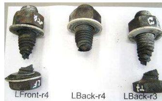
Figure 41: Bolts failed in test 7 (Left (L) connection, rows (r) 3 and 4)
