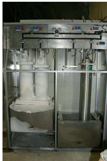
FIG. 4.10 – Xe recuperation system [41, 42]
