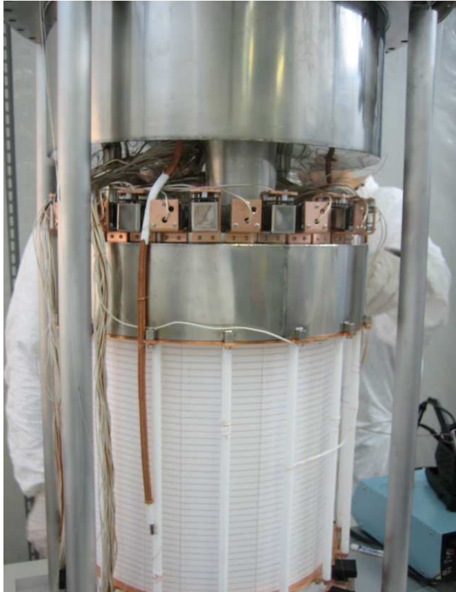
FIG. 4.3 – Teflon cylindrical structure of the detector [41, 42]
