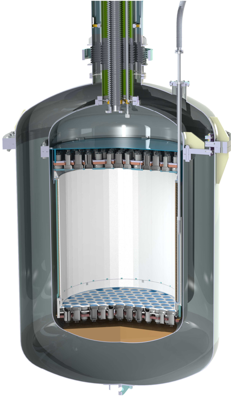
FIG. 6.2b — General inside view of the XENON1T TPC [68]
