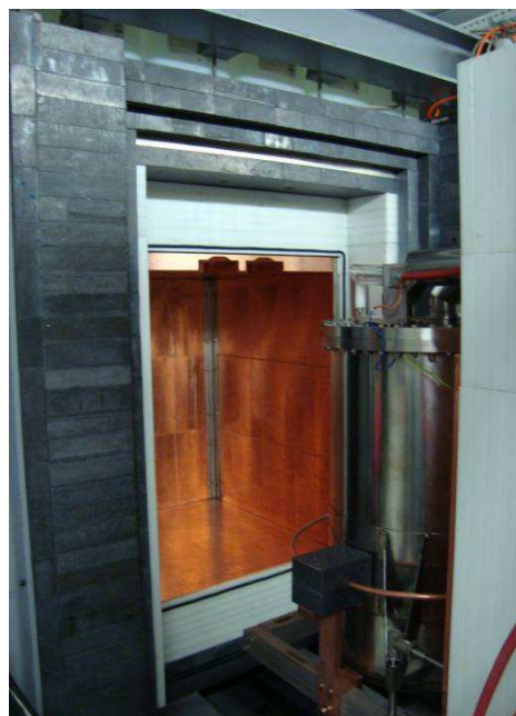
FIG. 4.7 – Image of water/ lead/ polyethylene/ copper shield [41, 42]
