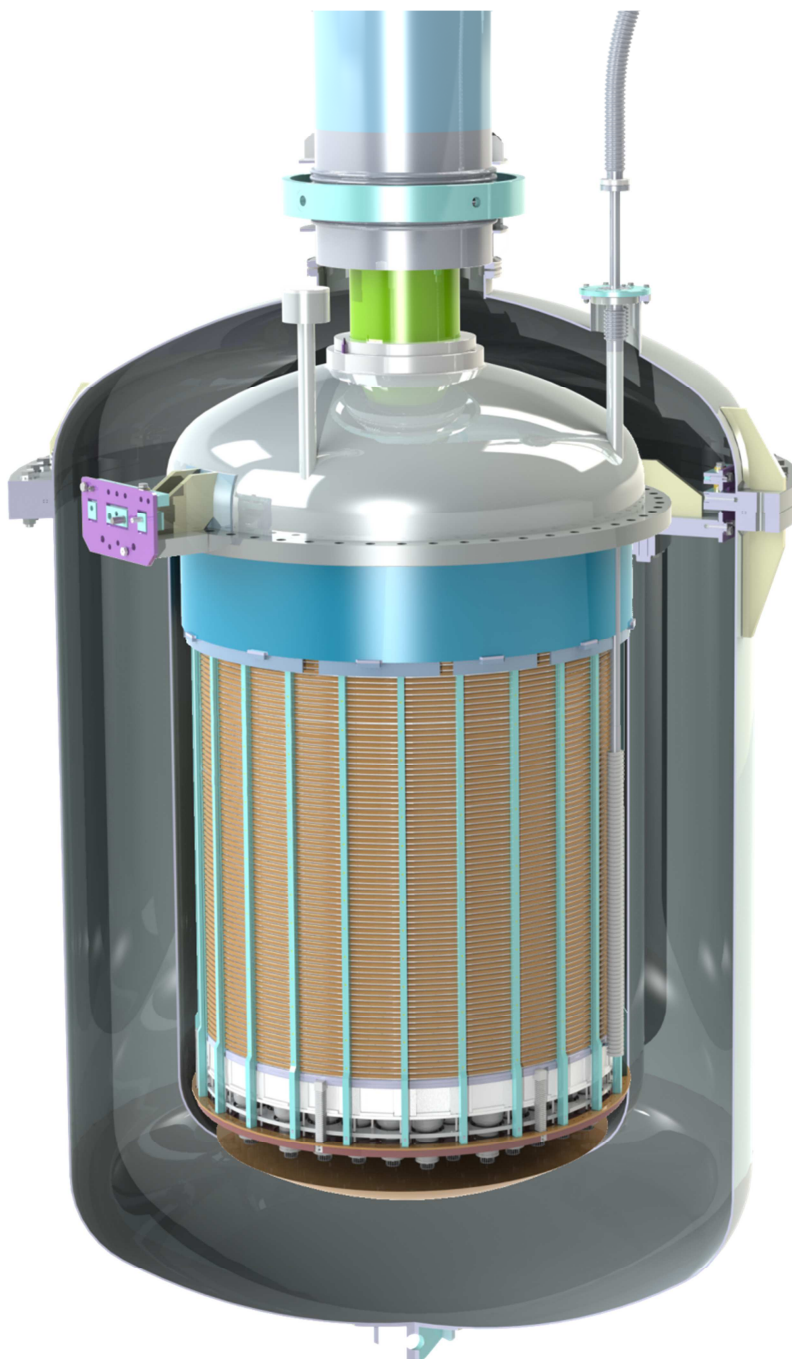
FIG. 6.2a – General outside view of the XENONIT TPC [68]
