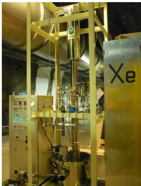
FIG. 4.9 – Kr purification system [41, 42]
