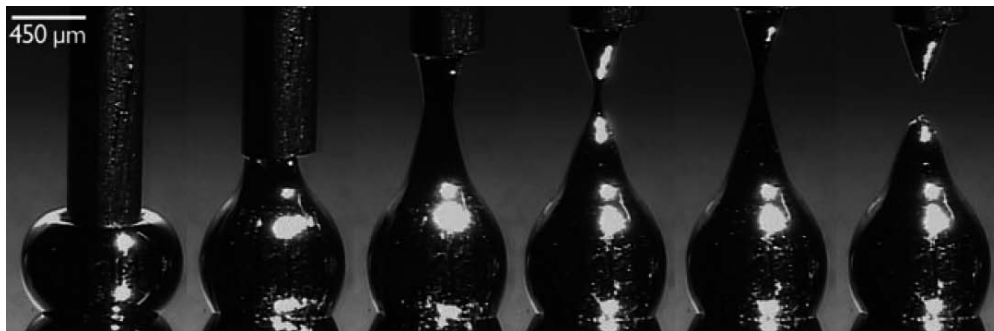
Figure 3.17: EGaIn drop: From left to right: The metal alloy suspended from a needle, brought into contact with a surface. At some point the material adheres to both of them. [39].
