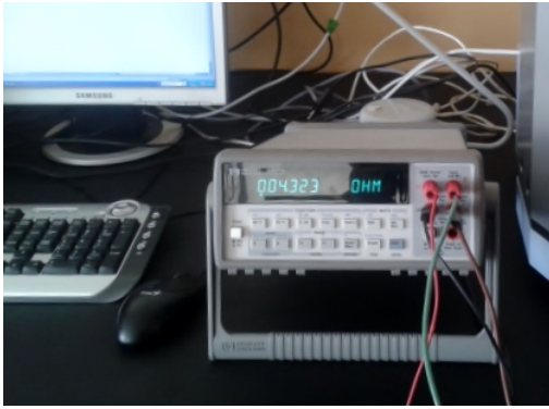
(a) Digital multimeter HP 34401A, using the 4-wire ohms method.
