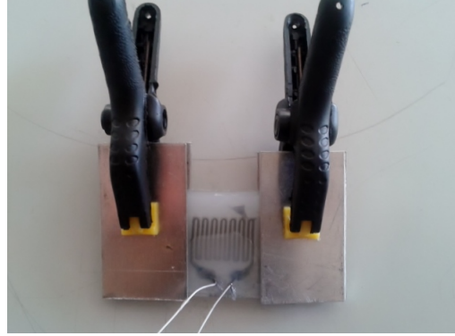
(b) Sensor fixed by two tweezers separated by a fixed distance of 23 mm.
