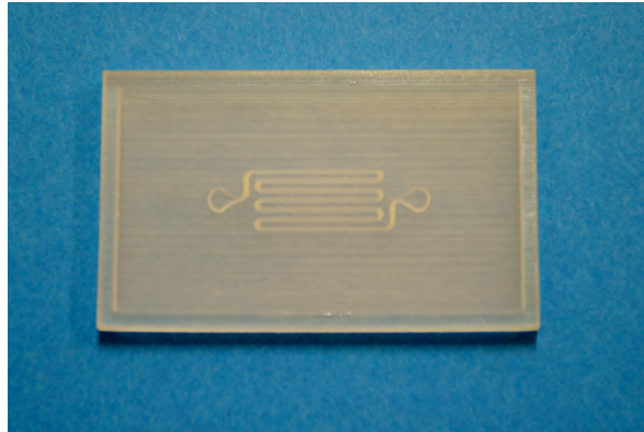
Figure 3.13: Mold for the third strain sensor printed with SLA Frosted Ultra Detail Plastic, matching the design shown in figure 3.6.
