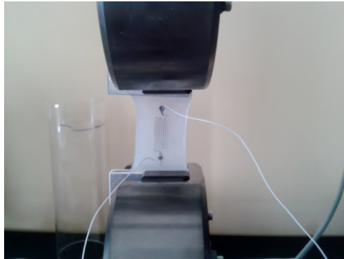
(c) Strain sensor in an universal testing Shimadzu AG-X to perform the x-axis strain test
