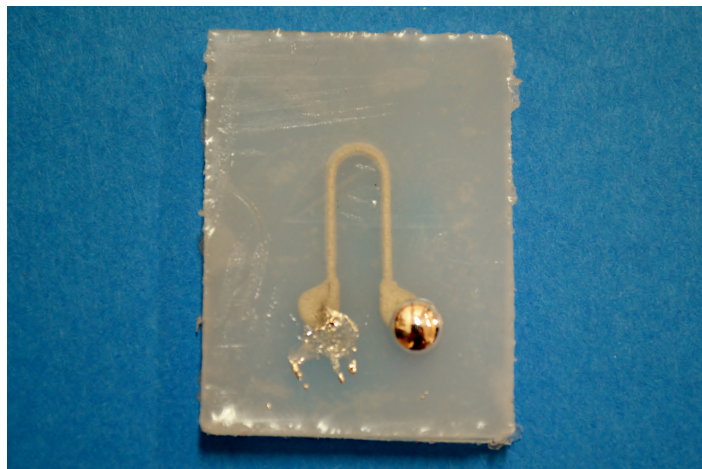
Figure 3.21: Example of metal coming off the sensor.
