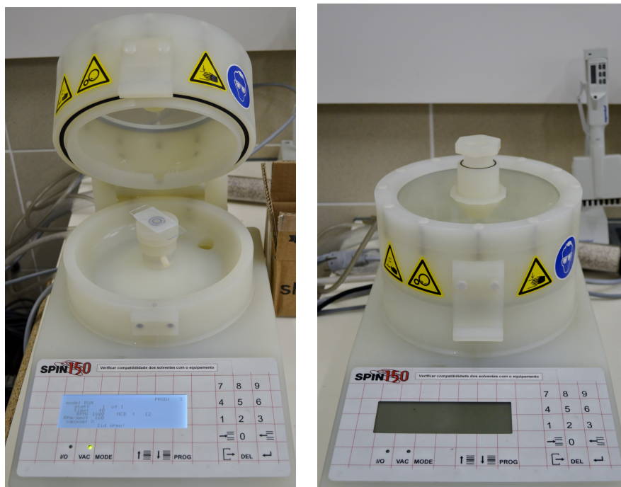
(a) Flat silicone layer placed on the spin-coater, with chosen parameters on the panel.
