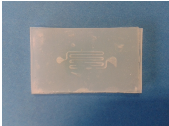
Figure 3.20: Example of blocked microchannels.
