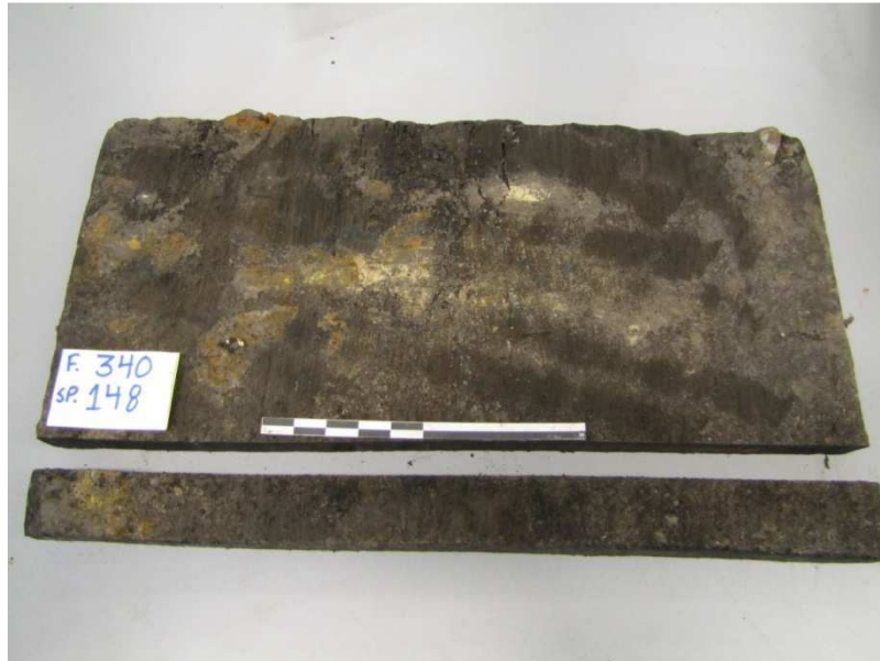
Figure 9. Sample sawn with a band-saw to obtain the transversal section of the plank (scale bar = 20 cm).
