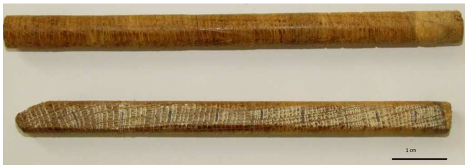
Figure 24. Two dry wood cores before (top) and after preparation (bottom). The lighter color on the right corresponds to the sapwood.
