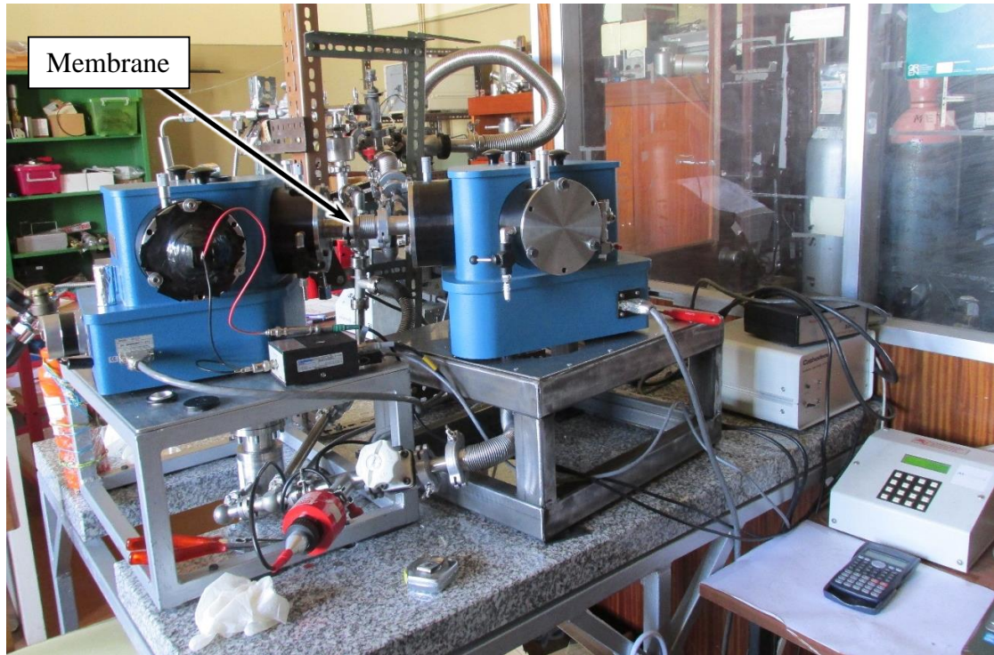
Figure 25: Photo of part of our experimental system, showing the two MCs, the main chamber, part of the data acquisition instrumentation and part of the vacuum system. The vacuum gauges and pumps are not visible.
