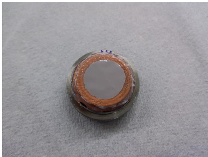
Figure 23: Uncoated membrane glued onto a copper support which is itself mounted on a vacuum system piece (center-ring support KF-25).
