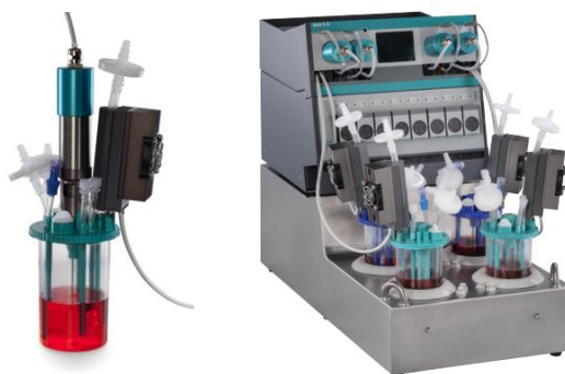
Figure 1.20 - A 4-fold DASbox® Mini Bioreactor System for cell culture. This system enables an on-line monitoring and control of specific cell culture parameters, such as temperature, pH, dissolved oxygen and nutrients. Adapted from http://www.dasgip.com/cell-culture/
