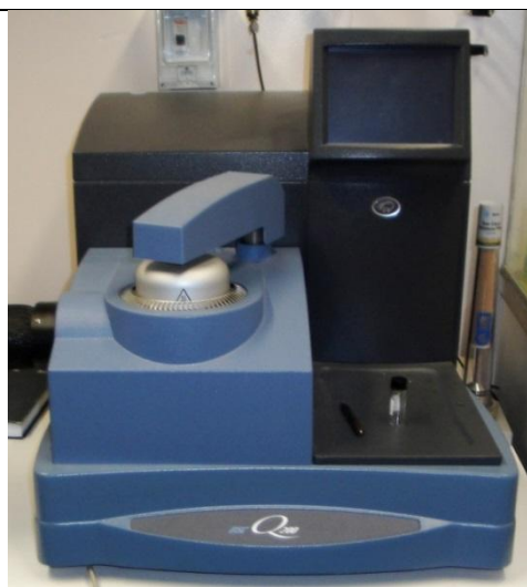
Figure 2.2 - Differential scanning calorimeter Model DSC Q200 (DSC)
