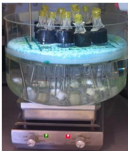
Figure 2.19 – Slow Stirring method, with samples at 25°C
