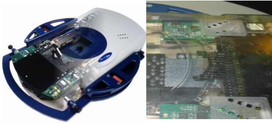
Figure 3.2 – m3 mMLC collimation system. Courtesy Brainlab.
