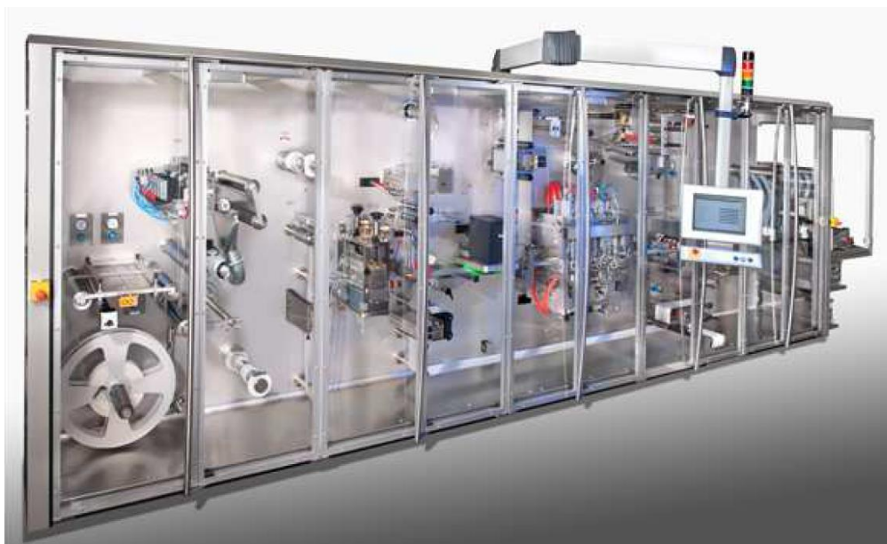
Figure 21 - Outlook of a pilot scale web converting and primary packaging machine (eq. P.D-P1).
