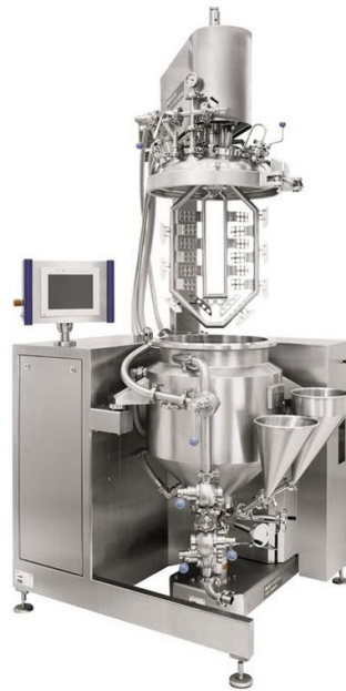
Figure 11 – Example of a mixing equipment with an anchor agitator. (Image from supplier M.A).
