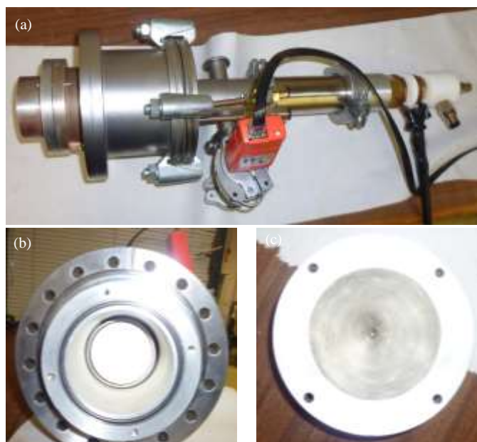
Figure 12 - (a) Clusters source, (b) inside view of the clusters source and (c) conical nozzle
