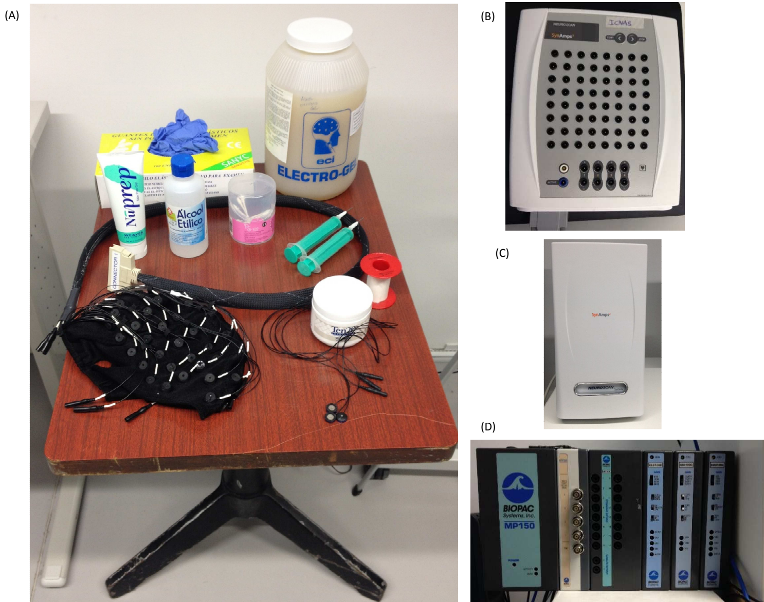
Figure A3. (A) Equipment required to perform EEG and EMG: gloves, swabs, alcohol, Nuprep, two 25 ml syringes, tape, EEG cap which connects to image B, EEG cap is filled with Electro-Gel, three EMG electrodes which connects to image D and EMG electrodes are filled with Ten20 conductive paste; (B) Head box which connects to EEG cap and image C; (C) NeuroScan amplifier which connects to the computer; (D) Biopac system used for EMG which connects to the computer.
