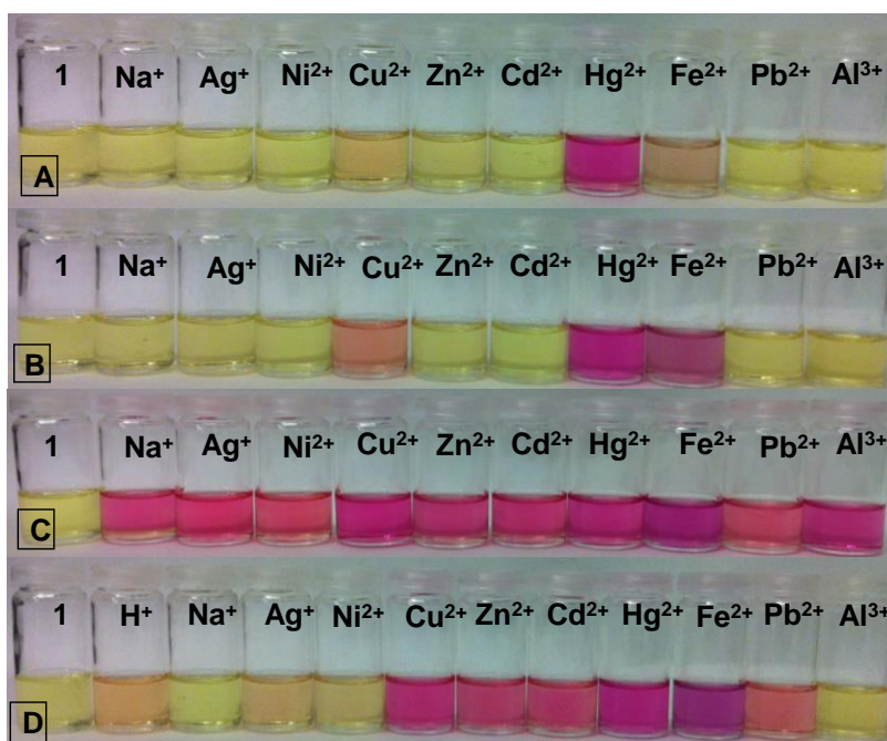
Picture 4.1. Naked-eye colorimetric behaviour of system 1 in four different conditions A to D. Condition A shows the naked eye colour solutions of 1 with the addition of one equivalent of metal ions; condition B with the addition of ten equivalents; condition C with the initial addition of ten equivalents and further addition of one equivalent of \text{Hg}^{2+} ; condition D with the initial addition of ten equivalents of metal ions and further addition of three equivalents of proton.
