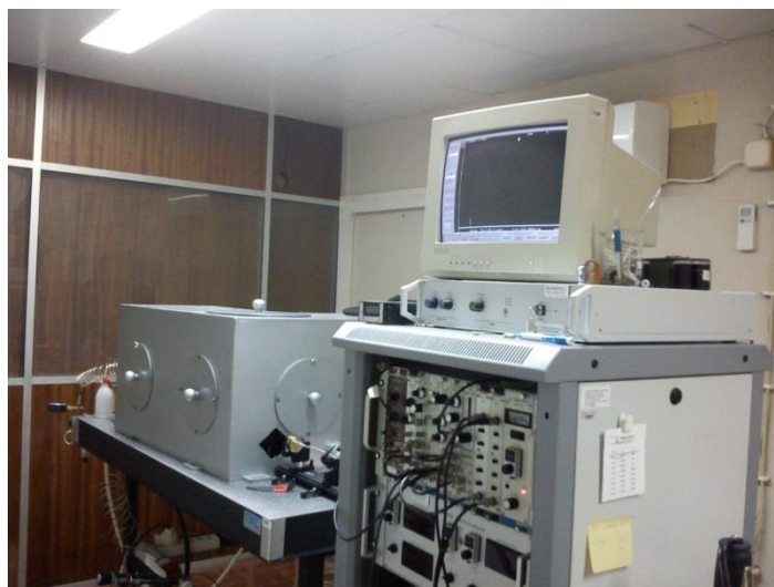
Figure 7.13. Picture of the ns-TCSPC apparatus used in this work.
