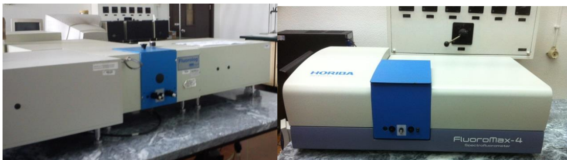
Picture 7.2. From left to right. Pictures of the Horiba-Jobin-Yvon SPEX Fluorolog 3-22 and Fluoromox-4 spectrofluorimetres used in these work.
