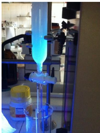
Figure 7.2. Photograph of the purification of 1-pyrenylmethyl methacrylate by silica column flash chromatography.
