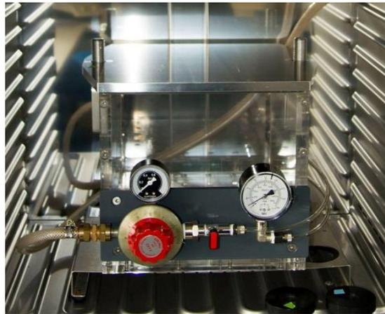
**Figure 12:** Pressure chamber used to expose cell cultures to elevated hydrostatic pressure (70 mmHg above atmospheric pressure)
