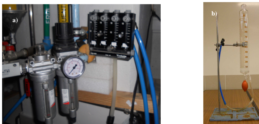
Figure 4.6: a) Air flow measuring system, b) home-made wet air flow meter.
