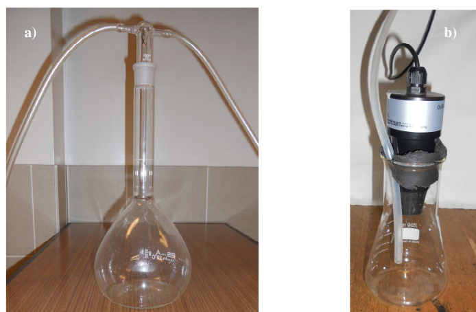
Figure 4.7: a) Water trap for the oxygen measuring system; b) oxygen gas sensor and measuring cell.
