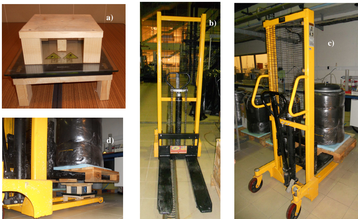
Figure 4.8: Reactor's weighing procedure: a) scale; b) pallet lift; c) raising of the reactor; d) reactor adjustment to the scale.
