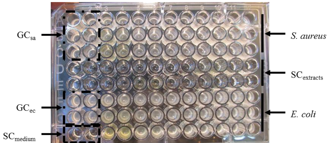
Figure 13. Microdilution assay performed to evaluate the antibacterial activity of O. pinnatifida extracts against S. aureus and E. coli (16-18h exposure, 35\pm 2^{\circ}\text{C} ). \text{GC}_{\text{sa}} – growth control wells of S. aureus (MHB + ultrapure water + microorganism); \text{GC}_{\text{ec}} – growth control wells of E. coli (MHB + ultrapure water + microorganism); \text{SC}_{\text{medium}} – sterility control wells of the culture medium (MHB alone); \text{SC}_{\text{extracts}} – sterility control wells for each tested extract concentration (MHB + extract + 0.85% saline).
