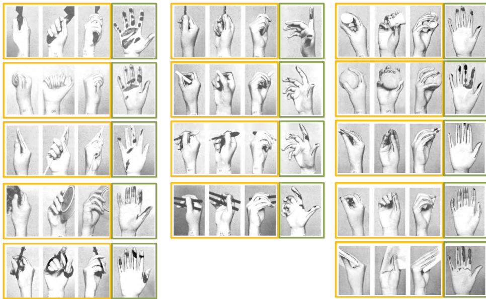
Figure 5.1: Schematic representation of the typical contact signatures of different grasps. Adapted from [Bernardin et al., 2005]. The boxes highlighted with orange border show different demonstrations of the grasp. The green border highlights the regions of the hand recruited to perform that type of grasp.
