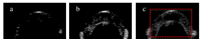
Fig. 2. B-scan images: (a) control lenses; (b) lenses with 60 minutes of immersion time; (c) lenses with 120 minutes of immersion time. Red line: region of interest for the texture analysis.
