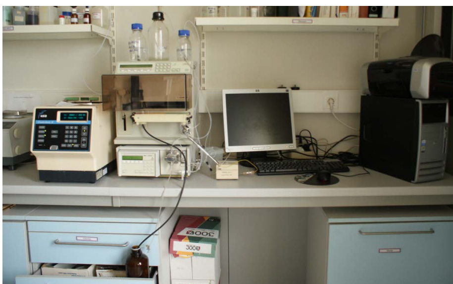
Figure 24: HPLC system used in this study for the quantification of monoamines.
