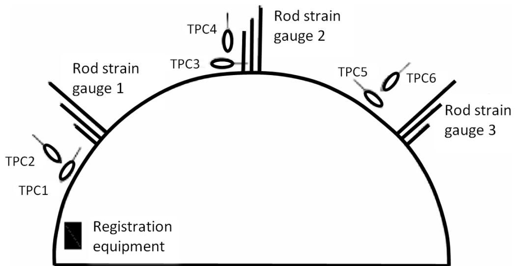
Fig. 3. Sketch of the cross-section monitoring arrangement. TPC - total pressure cell.
