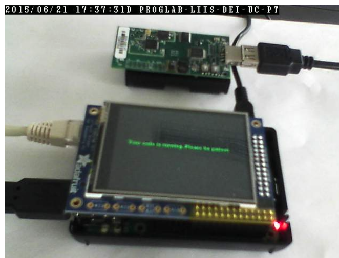
FIGURE 7.6: Camera view of the Remote Laboratory for Programming in Python.
