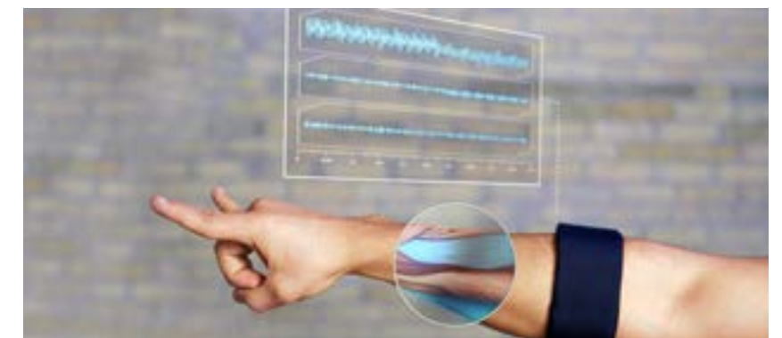
Figure 2.3 – MYO armband detects some gestures using electromyography signals (Picture credit: Thalmic Labs)
