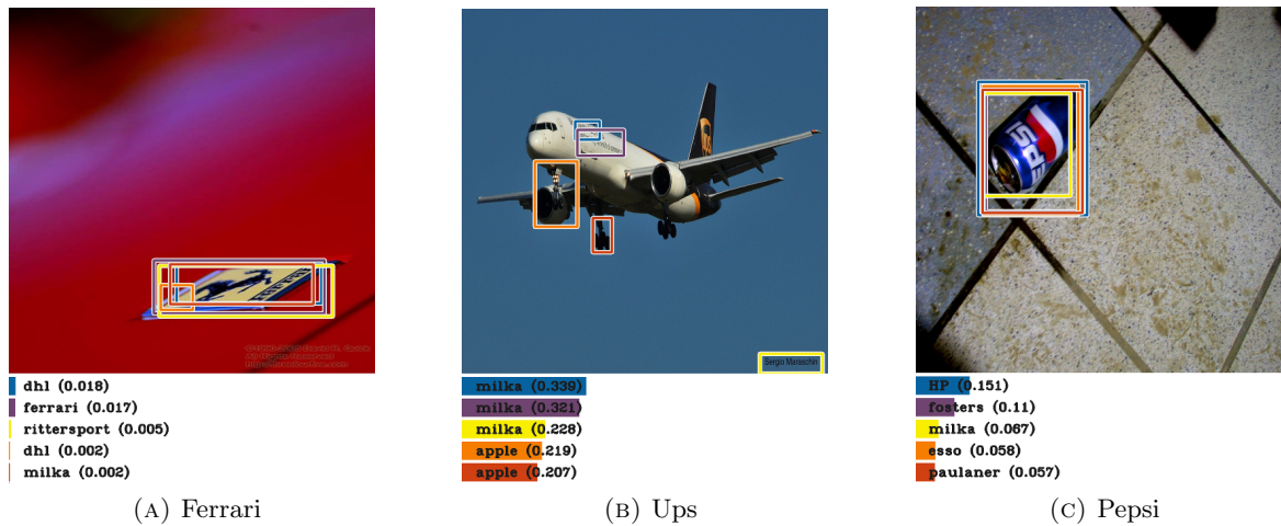
FIGURE 5.14: Graphic logos in slanted angles or partially occluded are not always correctly detected.
