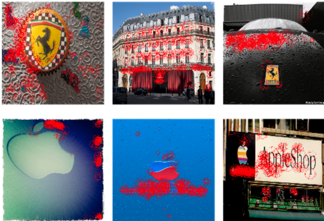
FIGURE 5.5: Regions for feature extraction selected by ORB in red. Note that most of the selected regions are background regions.
