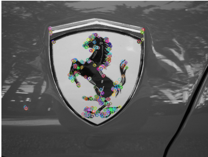
FIGURE 5.2: Keypoints detected in the image. Regions surrounding these points are selected for extraction, and then quantized.
