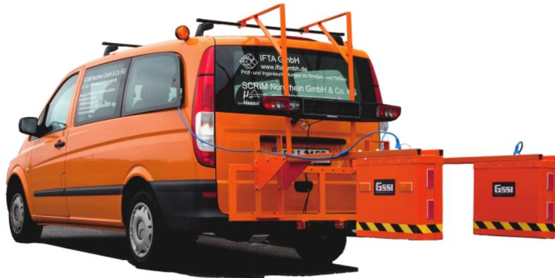
Figura 19: Ground penetrating radar
