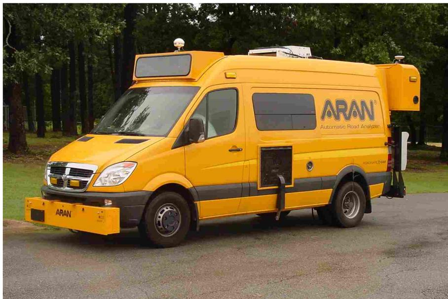
Figura 12: Automatic Road Aanalyser
