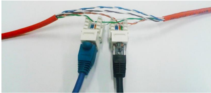
Figure 5-1 – Ethernet Tap using connectors attached to the Tx and Rx pairs
