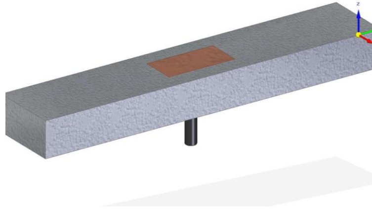
Figure 13: Integration of the electrodes in the internal surface of TPS. In black is shown the wire used for the signals transmission between the electrodes and the data acquisition unit.
