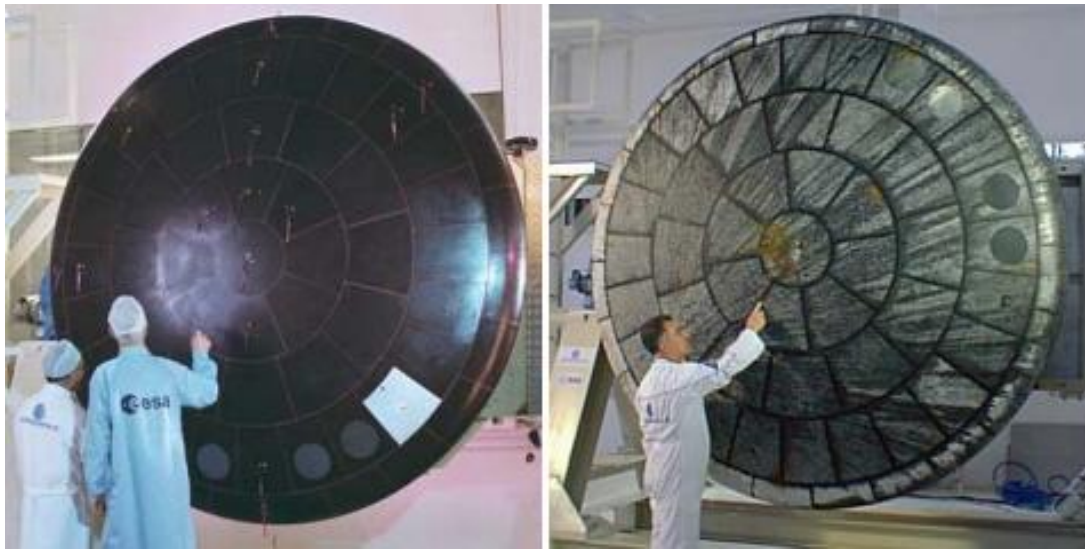
Figure 2: ARD Front-shield TPS a) before and b) after recovery [4].
