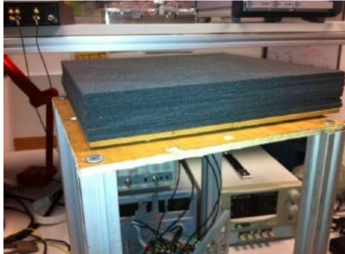
Figure 31: Testing TPIP response to thickness increase with Calcarb® layers. Note that the sensor is attached to a P50 plate with 5 mm thick [1].
