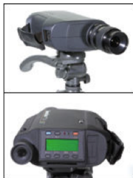
Figure 2. Colorimeter PR®-650 SpectraScan® (Topanga Canyon Place Chatsworth, CA) used in the experiment. Retrieved from: http://www.hometheater.com/content/ht-measurements-explained-rgb-triangle-death-video-measurements-page-2 .
