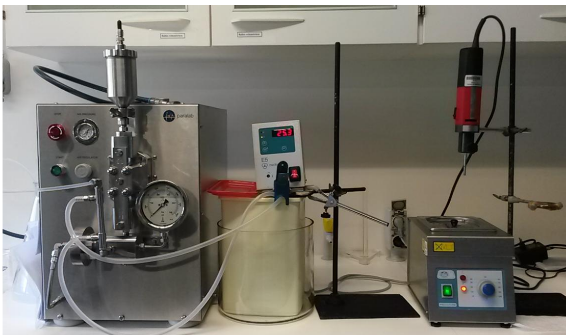
Figure 6: High pressure homogenizer (EmulsiFlex ® -C3, Avestin) and Ultra-Turrax ® , T25, IKA with the respective heating baths.
