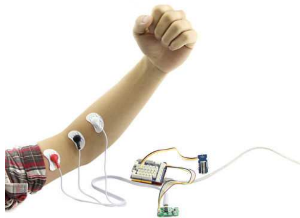
Figure 2.1 – EMG detector circuit with 3 electrodes placed on the forearm (Seeed Studio 2015)
