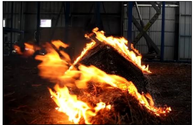
Fig 6-43 Image showing the extreme fire behavior on the down ridge direction and the height of the flame on the windward face, image from (3D18)
