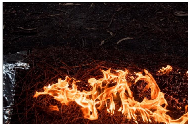
Fig 6-12 Image showing the fire front shape on the up ridge direction, image from (3D2)
