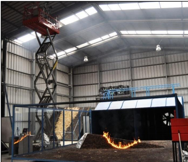
Fig 6-4 image showing the combustion wind tunnel and the model placed in its center, also the cameras are positioned on the left of the tunnel
