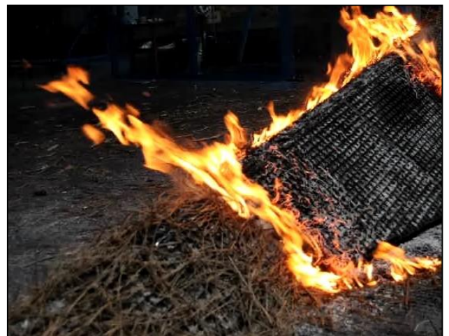
Fig 6-17 Image showing the intense fire behavior on the windward face caused by the wind sliding effect, image from (3D12)
