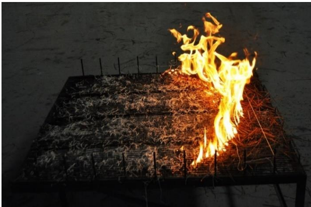
Fig 6-7 The 1 \text{ m}^2 area table where the R_o was defined
