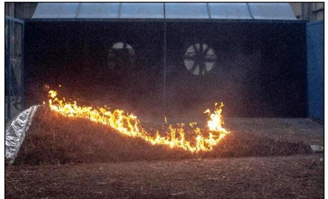
Fig 6-6A typical fire spread behavior on the leeward face (ref. 3D7)
