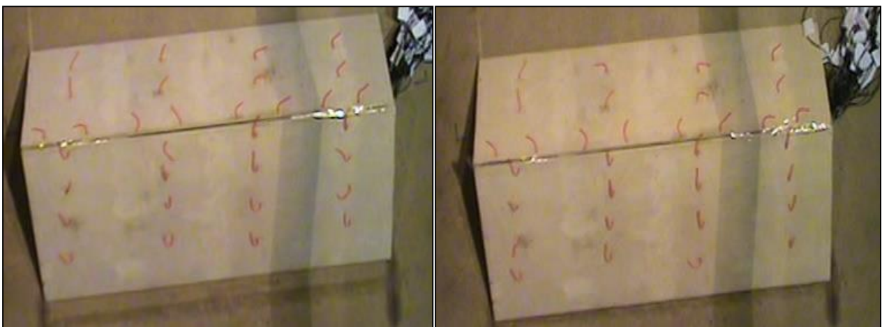
Fig 4-17 flow visualization for different tests for the 2D ridge ware conducted on the same wind tunnel
