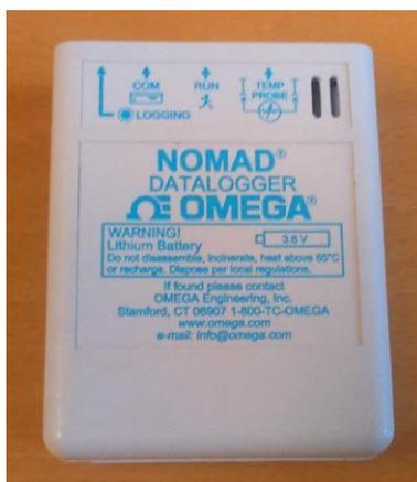
Figura 3-15. *Datalogger* Omega OM-NOMAD-RH-32
