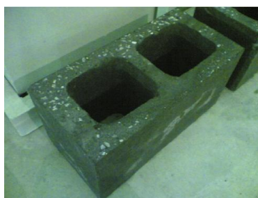
Figura 3.3 - Blocos ocios contendo grânulos de borracha (Mohammed et al, 2010)
