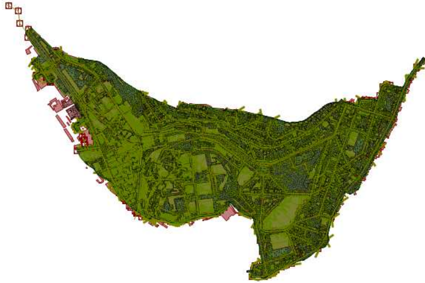
Figure 3.5 – 1D/2D semi-distributed dual drainage model used for the elaboration of the flood risk map
