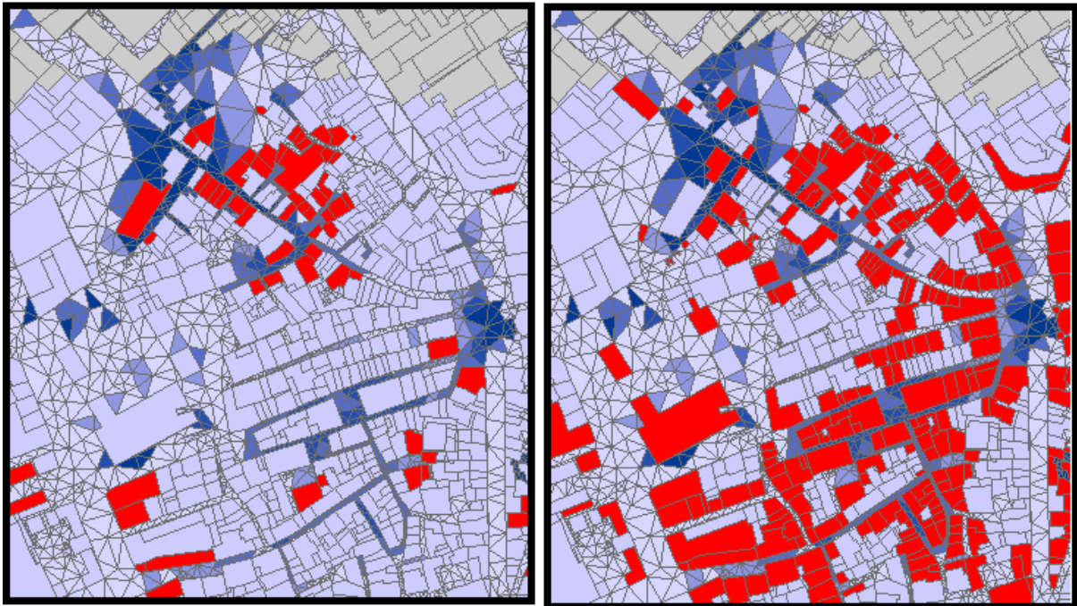
Figure 4.5 – Increase of buildings water depth classes, from return period of 20 to 50 years, and 50 to 100 years, respectively
