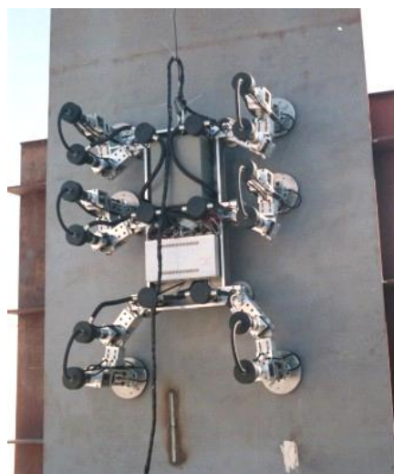
Figure 1.1 The REST , a climbing robot intended for welding in ferromagnetic walls. [2]
