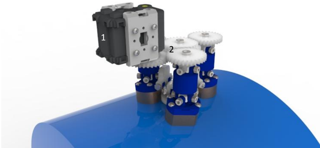
Figure 5.4 Transmission mechanism, with actuator (1) and transmission mechanism (2).
