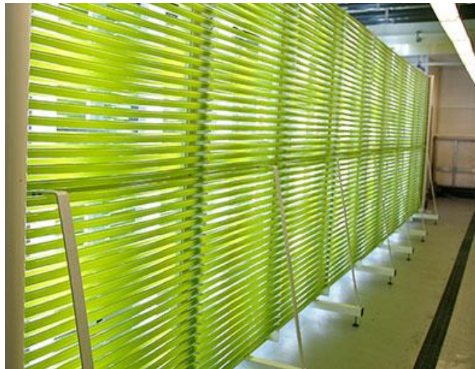
Figure 3 A commercial PBR set up at the NRC Institute for Marine Biosciences research station in Ketch Harbour, Nova Scotia ( www.chempuretech.com ).
