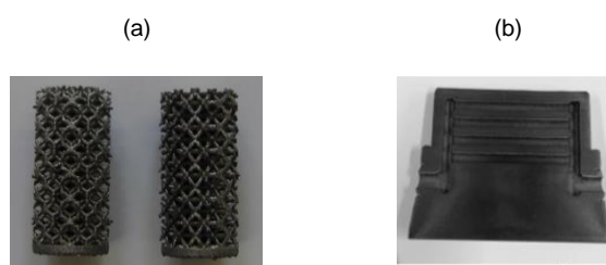
Figure. 7 – Alveolar structures and conformal channels.
