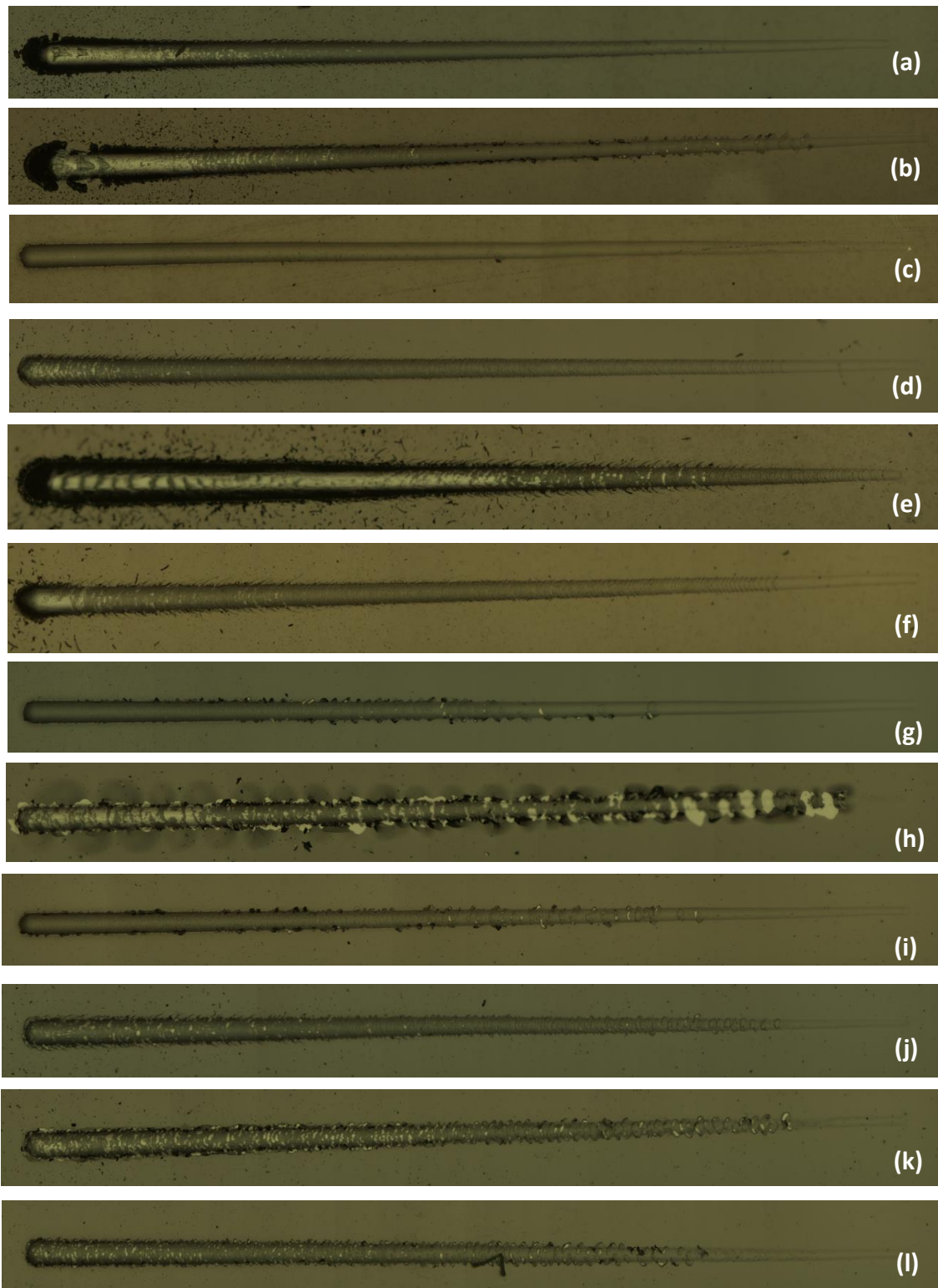
Figure 5.8. Scratch track morphologies of coatings in as deposited condition: a - c) and d to f) coatings containing 7 at.% Si deposited with low and high peak power, respectively. g to i) and j to l) coatings containing 12 at.% Si deposited with low and high peak power, respectively. (a) \text{TiSi}_7\text{N}_L , (b) \text{TiSi}_7\text{V}_6\text{N}_L , (c) \text{TiSi}_7\text{V}_{11}\text{N}_L , (d) \text{TiSi}_7\text{N}_H , (e) \text{TiSi}_7\text{V}_6\text{N}_H , (f) \text{TiSi}_7\text{V}_{11}\text{N}_H , (g) \text{TiSi}_{12}\text{N}_L , (h) \text{TiSi}_{12}\text{V}_6\text{N}_L , (i) \text{TiSi}_{12}\text{V}_{11}\text{N}_L , (j) \text{TiSi}_{12}\text{N}_H , (k) \text{TiSi}_{12}\text{V}_6\text{N}_H , and (l) \text{TiSi}_{12}\text{V}_{11}\text{N}_H
