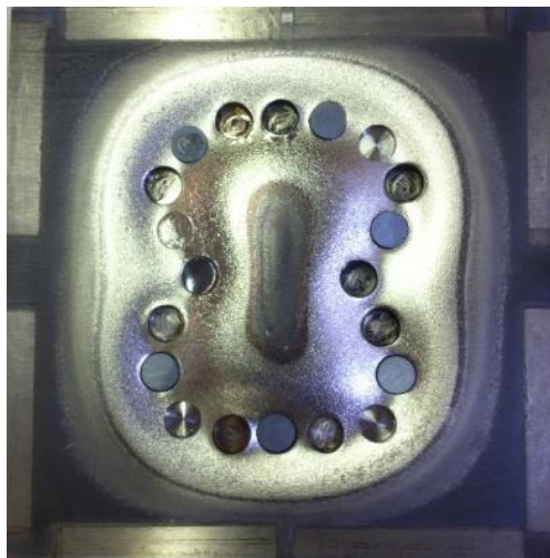
Figure 4.2. Ti target with 20 holes uniformly distributed throughout the preferential erosion zone and filled with Ti, Si and V pellets in different configurations
