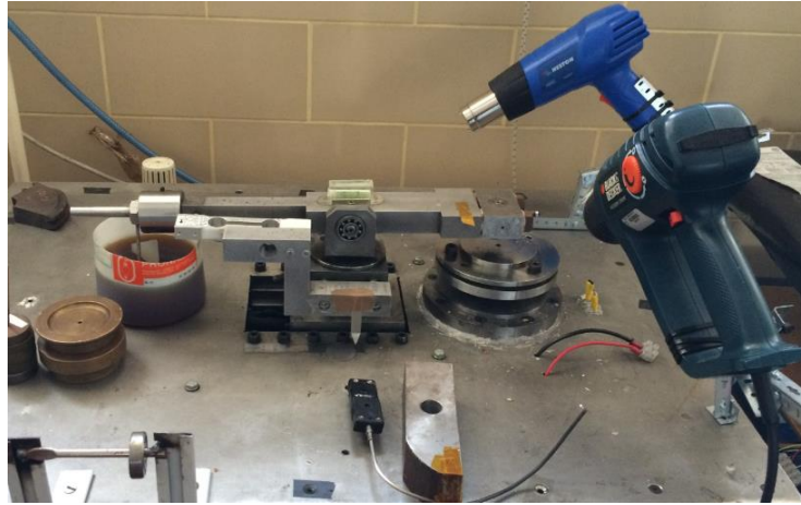
Figure 14 - The home-made pin-on-disk test rig used for studying the tribological behaviour of the coatings against rubber. The setup of the heating apparatus was done in a way to maintain the substrate surface temperature as close to the desired temperature as possible. The maximum temperature used for these tests was 200 °C.
