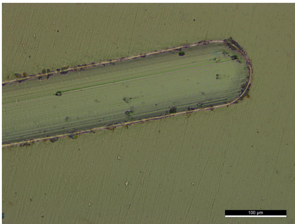
Appendix Fig 22 – Image of the adhesion test results on WSC49 (centre deposited) coating. The critical load was greater than 50 mN
