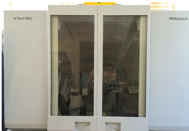
Figure 12 - The XRD setup used for this work.
