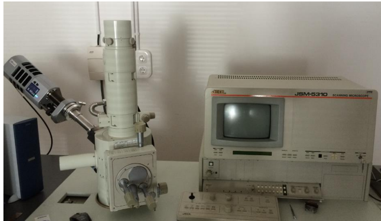
Figure 13 - The SEM instrument at IPN, LED & MAT used for studying the structure and the wear tracks of the coatings.
