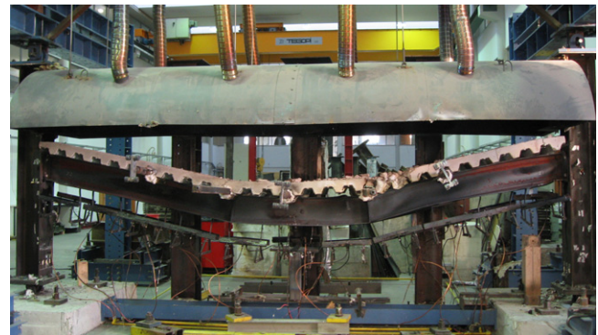
Fig. 30. Deformed structure after test FJ01.
