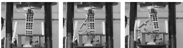
Fig. 16. Failure sequence of specimen PD2 3mm .
